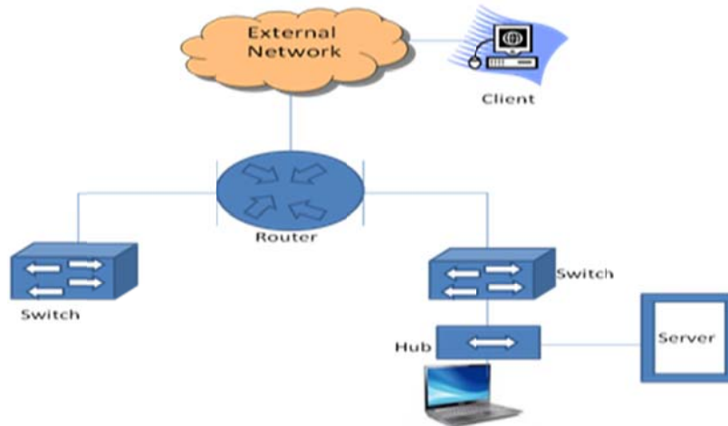
Figure 3. Wireshark placements using a Hub in an Institute
